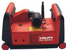
WALL CHASER - TRACK WALLS FOR CABLING
